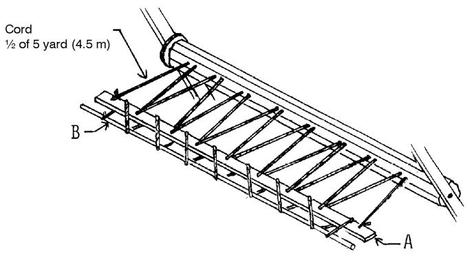
Cut the 5-yard (4.5 m) cord in half. One half of this cord laces beam stick A to warp rod B Insert a metal rod into the apron of the cloth beam. Use the other half of the cord to lace this rod to the third metal rod.
