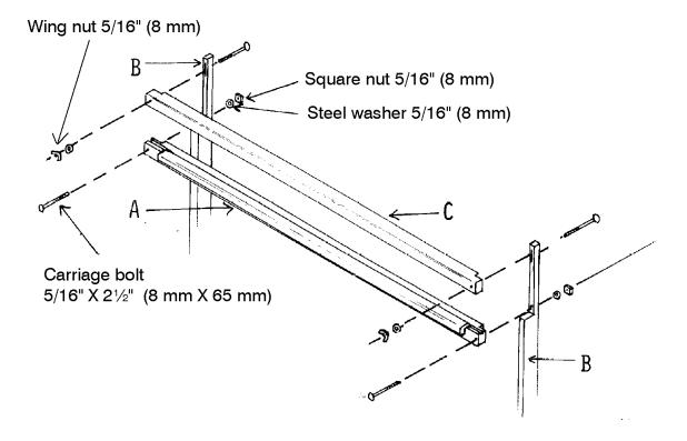
Using the carriage bolts, steel washers and square nuts, attach the batten sley A (with shuttle race) to the batten swords B.
