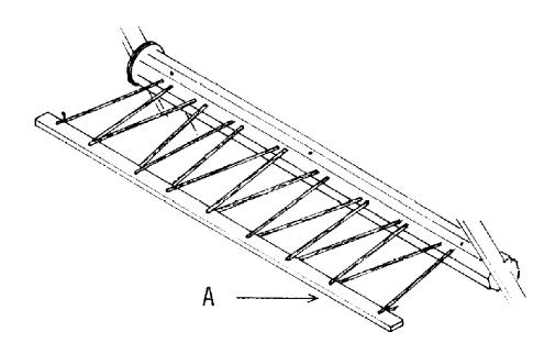
Continue threading the cord trought the warp beam and beam stick A. Knot the cord at each end of the beam stick.
