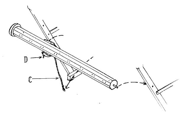
Unhook brake treadle cord C from the brake realease treadle.
