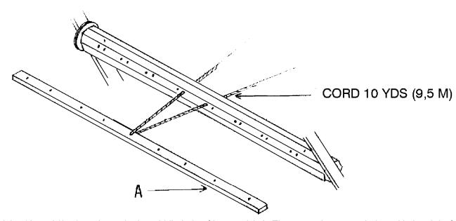
Thread the 10 yard (9 m) cord trought the middle hole of beam stick A. Then pass the two ends (equal in lenght) of this cord trought the niddle holes of the warp beam.
