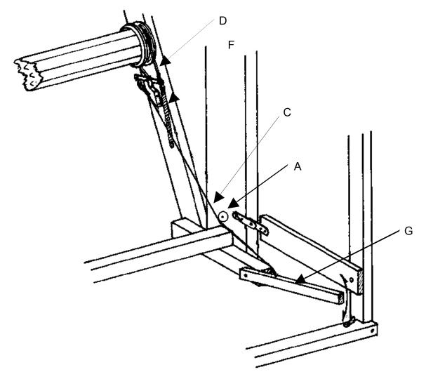
Attach the end of circular brake shoe D (wire brake circle) to the hook of spring F
