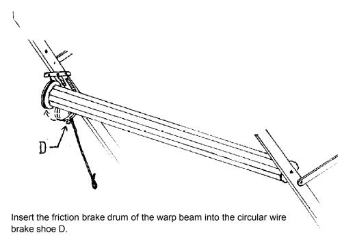
Do not unroll the brake shoe (brake circle), just slide the warp beam into it
