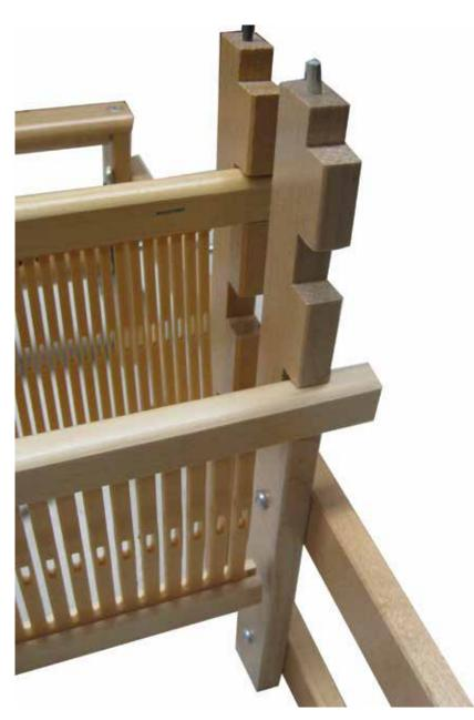
Install this new set of support 1" in front of the original one so you will be able to move up and down the rigid heddle.
