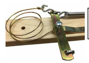
Use the screw no 12, 1 1/4" to install the lever, strengthning piece and brake circle assemble like in this picture.
