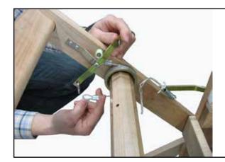
Unroll (unpack) the brake cable. Turn clockwise 3 times around the brake drum starting at the top.
