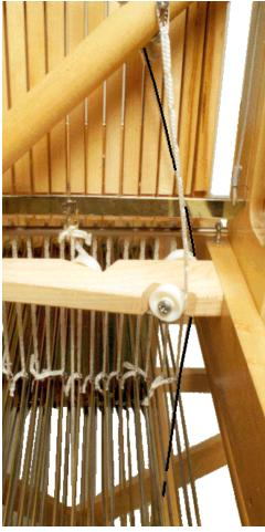
Install loop cord joining the screw hook of left treadle and hook under the knife, threading it between shaft frames. Adjust length so knife gets to the low position when the left treadle is depressed.
