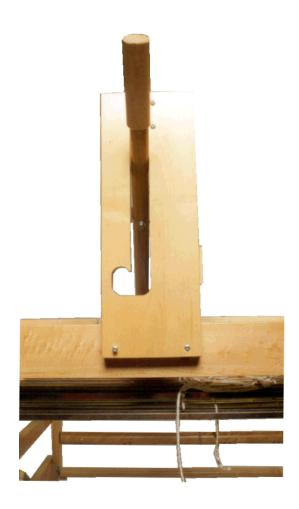
Install the shaft selector in place using 4 round head screws #8 - 1¼" Make sure to screw in the pre-drill holes. Make connection of the loop cord between the knife and the handle outside screw at black mark. Pass hole of black mark around the screw.
