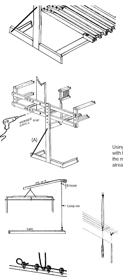
Screw the Upright post to the base using the 4 Carriage bolt ¼" x 1¾", 4 washers ¼" and 4 square nuts ¼"
