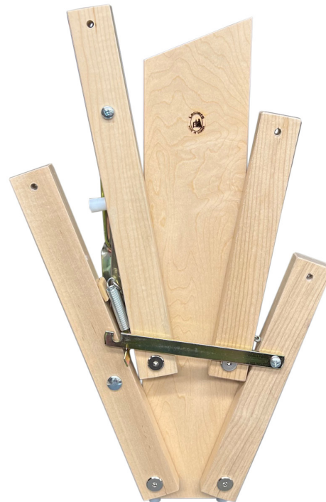
- Top board with shafts levers (#4)
