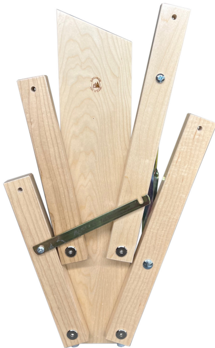
- Top board with shafts levers (#4)
