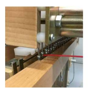
3- Spray into the ball bearing pulleys.
