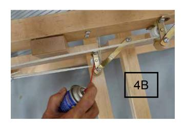
4- Spray in between the pulleys under the shaft frame. Treadle the loom a few times. Wipe off the excess silicone.
