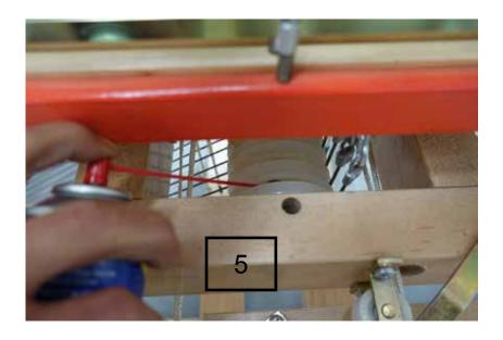
5- Once a year, spray between all the big pulleys. After spraying, treadle the loom several times.
