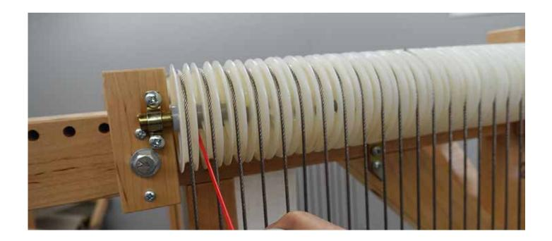
Note: Do not spray oil or silicone on the friction brake components.
